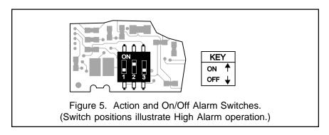
For newer models select the action by setting switch 1 on and switch 2 off (direct acting) or switch 1 off and switch 2 on (reverse acting). Switch 3 determines whether the output will reset after the temperature has moved to the other side of the set point. If switch 3 is on then the output will automatically reset. If switch 3 is off then the RESET button on the front of the control must be pushed before the output will reset.
