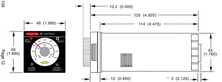
Panel cutout for all models is  $45 \text{mm} \times 45 \text{mm} \times 1.775 \text{in}$ . Allow for  $13 \text{mm} \times (0.5 \text{in})$  clearance at the rear.
