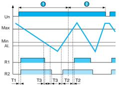
On power-up, probes Min, Max and AI. are submerged, relays R1 and R2 are energised and the pump is ON : emptying starts, the LED for relay R1 is lit. When the Min probe emerges, relay R1 goes off. If, in the event of a fault, the level continues to fall and probe AI. emerges, relay R2 deenergises and the alarm is triggered : the LED relay R2 is lit. This fault can be stored.
