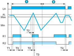
On power-up, probes Min, Max are submerged and probe AI. is above the level of the liquid. Relays R1 and R2 are energised and the pump is ON : emptying starts, the LED for relay R1 is lit. When the Min probe emerges, relay R1 de-energises and the pump if OFF : emptying stops, the LED for relay R1 goes off. If, in the event of a fault, the level continues to rise and reaches proble AI., relay R2 de-energises and the alarm is triggered : the LED for relay R2 is lit.
